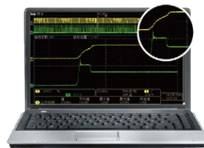
Fast voltage built with turn-on over range inrush current (CV-High, CC-Low, CV takes precedence)
