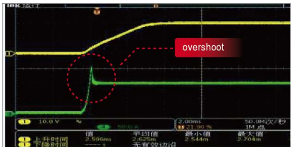
Diode load Conventional power test
