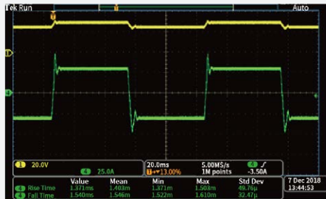
Control loop CV priority mode
