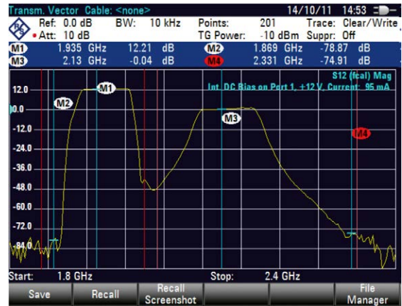
Two-port capability for transmission measurements
