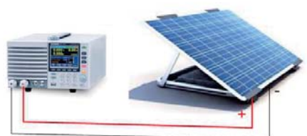
Connections Between PEL-3041 and Solar Panel
