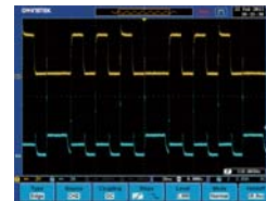
Voltage and Current Waveforms of the Receiving Signals of a Cellular Phone
