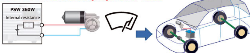
PSW Built-in Resistance Variable Function Simulating Battery Output Resistance and Wire Harness
