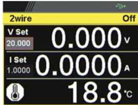
White: Temperature Control on with GTL-205A Connected
