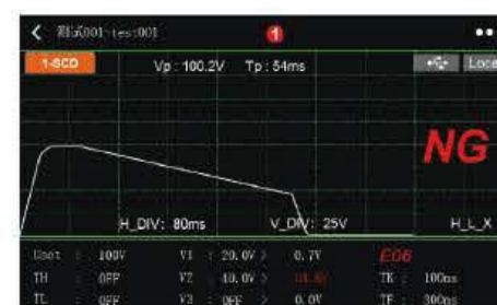
Figure 1/2 Test process of qualified and unqualified 5uF battery cell under 100V voltage (voltage rise time 54ms)
