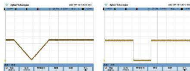
Simulation Battery Slow Drop and Slow Rise Supply Voltage Test
