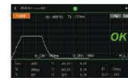
Figure 2 Test process of 40uF battery cell under 400V voltage (boosting time 122ms)
